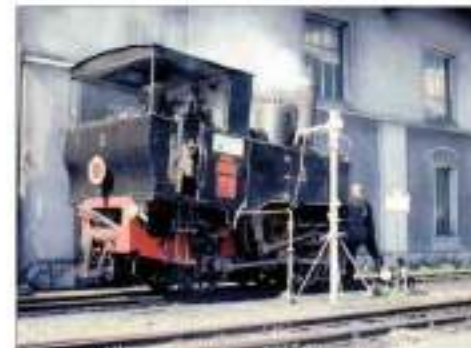
23. The water is pumped into the engines by a steam pump powered by a tap to the boiler. Rack locomotives have their water levels read in the center of the boiler or (the side tanks because the readings would otherwise be accurate only if the engine were on level ground. The water glass is out view above the three-gauge cocks on #3's side tank.
