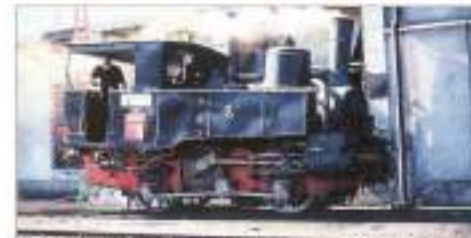
22. #3 has her bunker filled with coal from the modern cooling tower. Although Achenseebahn is proud to be a traditional steam rack railroad, Ing. Berhard Marchi has made some improvements such as this, based on the experience he gained as a fireman and locomotive engineer. In those days, this job was done by hand. Achenseebahn #3, Jenbach, Austria, August 14, 2000.
