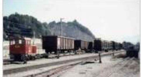
9. D-12 is spotting an inbound train for unloading the empty ÖBB cars. To the right of the cut is an outbound train of loaded cars, and at the far right is a pit track used for loading or unloading narrow gauge equipment on to, or off of, standard gauge flatcars, which are loaded on narrow gauge transporter wagons.
