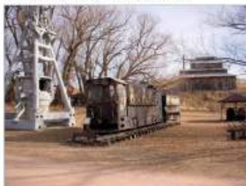
This Engine photo is an electric trammer called a loci. It was used to haul ore between the Henderson mine and, (I believe,) Empire, CO. Photo courtesy WMMI, caption Dave Futey, WMMI.
