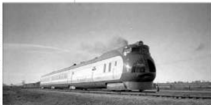
The photos above show the UP -M10,000, The Union Pacific Railroad's M-10000, delivered to the railroad on February 12, 1934, at a cost of $230,997, was the first internal combustion engine, lightweight streamlined express passenger train in the United States. The car bodies and interior fittings were built by Pullman-Standard. The 600 hp (450 kW) V12 distillate engine was from General Motors' Cleveland subsidiary, the Winton Engine Company — not, as is usually reported, the Electro-Motive Corporation, which merely supervised installation of the engine into the Pullman-built body. This engine design was not related to the later 201 or 201A Winton diesels. As for EMC, being primarily a marketing organization at this time, it did not manufacture any component parts of the M-10000. The air brake compressor, main generator, traction motors and control equipment were manufactured by the General Electric Company.
